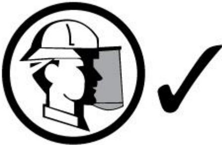
Correct application of reversed hard hat with nape strap at back of head
