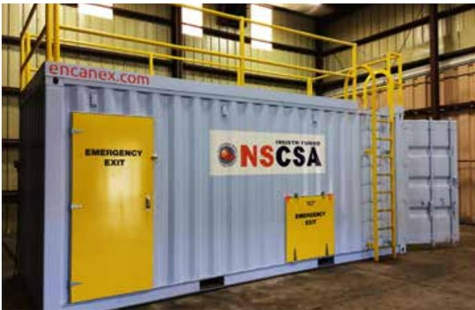
Construction Safety NS's confined space simulator
